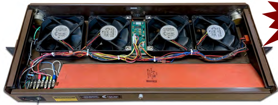
REFURBISHED DMS OPM, NT8X06AB FAN TRAY * WITH (4) NEW 48V FANS & NEW ALARM CONTROL BOARD
